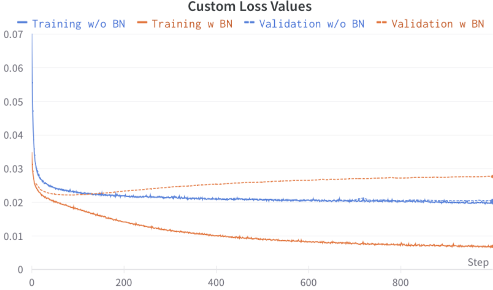
Figure 5: Loss values recorded for the 'vanilla' model w and w/o Batch Normalization layers, using a learning rate of 5 \times 10^{-5} and the custom loss function.
